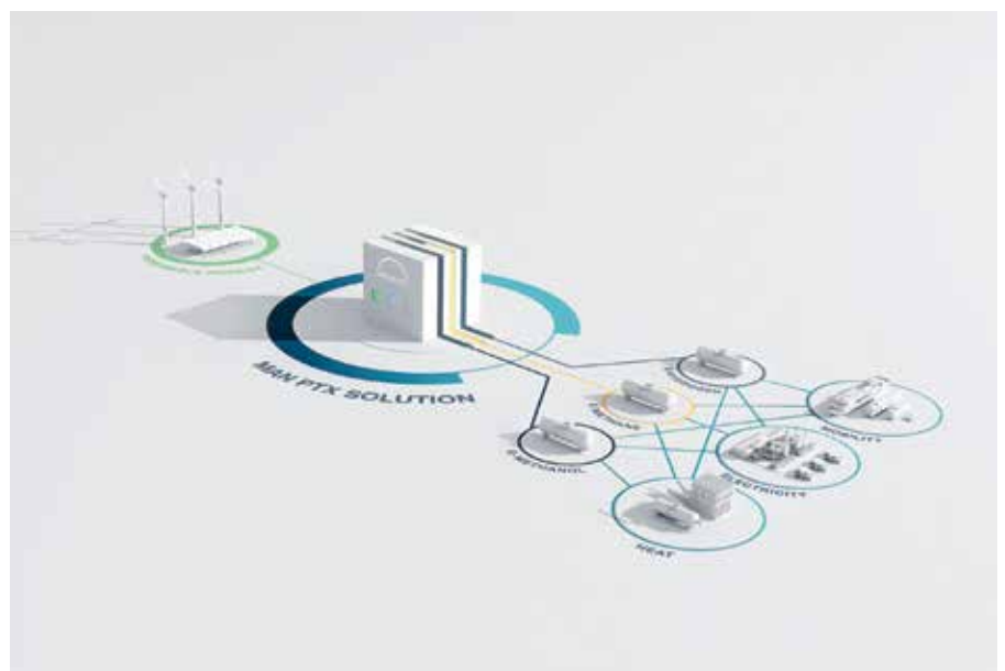
Fig. 3: Production of green NH 3 by harvesting energy from renewable sources and using it to produce H 2 from water via electrolysis and N 2 via liquefaction of air
